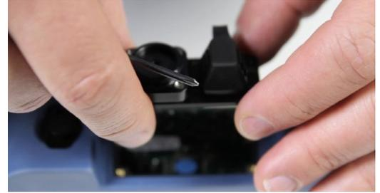
The power meter and VFL piece are offered as an easy-to-install option on the MAX-FIP display that's as simple removing four screws.
